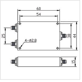
RF Solution offer a wide selection of 2 Ways Power Divider for global customers. PD02-F4460-S-698-6000MHz is a 2 Ways Power Divider in Frequency Range of 698~6000 MHz. It is made of high quality materials under a high standard, the Insertion Loss Max of this product is 1.5 dB, Split Loss is 3.0 dB and Isolation Min is 18 dB. The component has a good working performance and stability, it is ideal for handling a Rated Power of 50 W.
