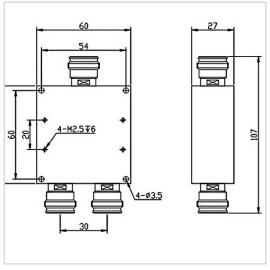
RF Solution offer a wide selection of 2 Ways Power Divider for global customers. PD02-F6066-M-698-4000MHz is a 2 Ways Power Divider in Frequency Range of 698~4000 MHz. It is made of high quality materials under a high standard, the Split Loss of this product is 3.0 dB, Insertion Loss Max is 0.8 dB and Isolation Min is 20.0 dB. The component has a good working performance and stability, it is ideal for handling a Rated Power of 50 W.
