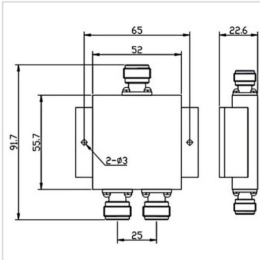
RF Solution offer a wide selection of 2 Ways Power Divider for global customers. PD02-F6556-N-2.4-2.5GHz is a 2 Ways Power Divider in Frequency Range of 2.4~2.5 GHz. It is made of high quality materials under a high standard, the Insertion Loss Max of this product is 0.5 dB, Isolation Min is 20 dB and Split Loss is 3.5 dB. The component has a good working performance and stability, it is ideal for handling a Forward Power of 50 W.
