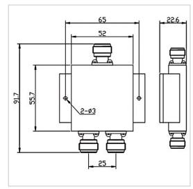
RF Solution offer a wide selection of 2 Ways Power Divider for global customers. PD02-F6556-N-4.8-5.2GHz is a 2 Ways Power Divider in Frequency Range of 4.8~5.2 GHz. It is made of high quality materials under a high standard, the Insertion Loss Max of this product is 0.3 dB, Isolation Min is 25 dB and Split Loss is 3.5 dB. The component has a good working performance and stability, it is ideal for handling a Rated Power of 50 W.
