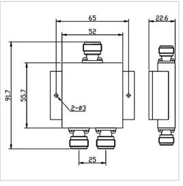
RF Solution offer a wide selection of 2 Ways Power Divider for global customers. PD02-F6556-N-5.15-5.85GHz is a 2 Ways Power Divider in Frequency Range of 5.15~5.85 GHz. It is made of high quality materials under a high standard, the Insertion Loss Max of this product is 0.5 dB, Isolation Min is 20 dB and Split Loss is 3.5 dB. The component has a good working performance and stability, it is ideal for handling a Rated Power of 50 W.
