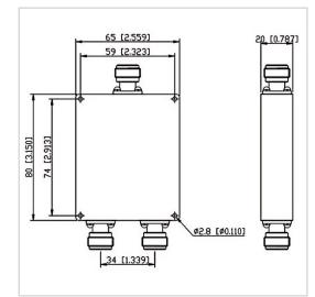
RF Solution offer a wide selection of 2 Ways Power Divider for global customers. PD02-F6580-N-100-1000MHz is a 2 Ways Power Divider in Frequency Range of 100~1000 MHz. It is made of high quality materials under a high standard, the Split Loss of this product is 3.0 dB, Insertion Loss Max is 1.0 dB and Isolation Min is 20.0 dB. The component has a good working performance and stability, it is ideal for handling a Forward Power of 30 W.
