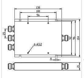
RF Solution offer a wide selection of 3 Ways Power Divider for global customers. PD03-F1013-N-698-3800MHz is a 3 Ways Power Divider in Frequency Range of 698~3800 MHz. It is made of high quality materials under a high standard, the Insertion Loss Max of this product is 1.2 dB, Isolation Min is 20 dB and Split Loss is 4.8 dB. The component has a good working performance and stability, it is ideal for handling a Rated Power of 50 W.
