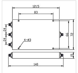
RF Solution offer a wide selection of 3 Ways Power Divider for global customers. PD03-F7212-S-698-3800MHz is a 3 Ways Power Divider in Frequency Range of 698~3800 MHz. It is made of high quality materials under a high standard, the Insertion Loss Max of this product is 1.2 dB, Isolation Min is 20 dB and Split Loss is 4.8 dB. The component has a good working performance and stability, it is ideal for handling a Rated Power of 50 W.
