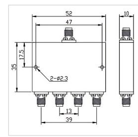
RF Solution offer a wide selection of 4 Ways Power Divider for global customers. PD04-F5235-S-18-40GHz is a 4 Ways Power Divider in Frequency Range of  $18.0 \sim 40.0$  GHz. It is made of high quality materials under a high standard, the Insertion Loss Max of this product is 1.8 dB, Isolation Min is 16 dB and Amplitude Unbalance is  $\pm 0.4$  dB. The component has a good working performance and stability, it is ideal for handling a Forward Power of 10 W.
