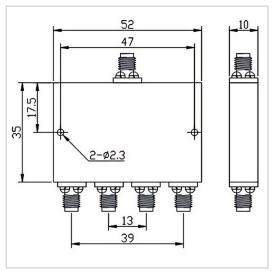
RF Solution offer a wide selection of 4 Ways Power Divider for global customers. PD04-F5235-S-6-40GHz is a 4 Ways Power Divider in Frequency Range of  $6.0\sim40.0$  GHz. It is made of high quality materials under a high standard, the Insertion Loss Max of this product is 1.8 dB, Isolation Min is 16 dB and Amplitude Unbalance is  $\pm0.4$  dB. The component has a good working performance and stability, it is ideal for handling a Forward Power of 10 W.
