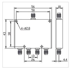
RF Solution offer a wide selection of 4 Ways Power Divider for global customers. PD04-F5643-S-1-4GHz is a 4 Ways Power Divider in Frequency Range of  $1.0{\sim}4.0$  GHz. It is made of high quality materials under a high standard, the Insertion Loss Max of this product is 0.8 dB, Isolation Min is 20 dB and Amplitude Unbalance is  $\pm 0.3$  dB. The component has a good working performance and stability, it is ideal for handling a Forward Power of 30 W.
