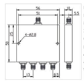
RF Solution offer a wide selection of 4 Ways Power Divider for global customers. PD04-F5650-S-2-4GHz is a 4 Ways Power Divider in Frequency Range of 2.0~4.0 GHz. It is made of high quality materials under a high standard, the Insertion Loss Max of this product is 0.8 dB, Isolation Min is 20 dB and Amplitude Unbalance is  $\pm$ 0.3 dB. The component has a good working performance and stability, it is ideal for handling a Forward Power of 30 W.
