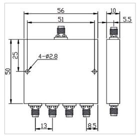
RF Solution offer a wide selection of 4 Ways Power Divider for global customers. PD04-F5650-S-2-8GHz is a 4 Ways Power Divider in Frequency Range of  $2.0{\sim}8.0$  GHz. It is made of high quality materials under a high standard, the Insertion Loss Max of this product is 1.0 dB, Isolation Min is 20 dB and Amplitude Unbalance is  $\pm 0.4$  dB. The component has a good working performance and stability, it is ideal for handling a Forward Power of 30 W.
