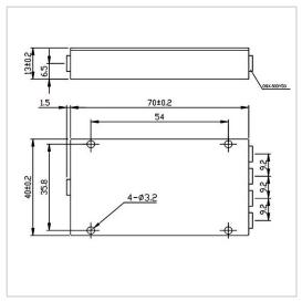
RF Solution offer a wide selection of 4 Ways Power Divider for global customers. PD04-F7040-O-950-4000MHz is a 4 Ways Power Divider in Frequency Range of 950~4000 MHz. It is made of high quality materials under a high standard, the Insertion Loss Max of this product is 7.5 dB, Isolation Min is 18 dB and Amplitude Balance Max is 0.5 dB. The component has a good working performance and stability, it is ideal for handling a Rated Power of 10 W.
