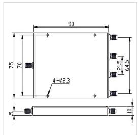
RF Solution offer a wide selection of 4 Ways Power Divider for global customers. PD04-F7590-S-1-12.4GHz is a 4 Ways Power Divider in Frequency Range of  $1.0 \sim 12.4$  GHz. It is made of high quality materials under a high standard, the Insertion Loss Max of this product is 2.8 dB, Isolation Min is 16 dB and Amplitude Unbalance is  $\pm 0.5$  dB. The component has a good working performance and stability, it is ideal for handling a Forward Power of 20 W.
