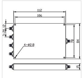
RF Solution offer a wide selection of 4 Ways Power Divider for global customers. PD04-F8411-S-698-6000MHz is a 4 Ways Power Divider in Frequency Range of 698~6000 MHz. It is made of high quality materials under a high standard, the Insertion Loss Max of this product is 1.8 dB, Isolation Min is 18 dB and Split Loss is 6.0 dB. The component has a good working performance and stability, it is ideal for handling a Rated Power of 50 W.
