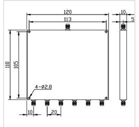
RF Solution offer a wide selection of 6 Ways Power Divider for global customers. PD06-F1211-S-700-3000MHz is a 6 Ways Power Divider in Frequency Range of 700~3000 MHz. It is made of high quality materials under a high standard, the Insertion Loss Max of this product is 1.6 dB, Isolation Min is 20 dB and Amplitude Unbalance is  $\pm 0.1$  dB. The component has a good working performance and stability, it is ideal for handling a Forward Power of 30 W.
