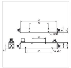
RF Solution offer a wide selection of Coupler for global customers. PD06-F1585-S-0.698-2.7GHz is a Coupler in Frequency Range of 0.698~2.7 GHz. It is made of high quality materials under a high standard, the Insertion Loss Max of this product is 0.65 dB , Nominal Coupling is  $6\pm 1$  dB and Coupling Sensitivity Max is  $\pm 0.8$  dB. The component has a good working performance and stability, it is ideal for handling a Rated Power of 50 W.
