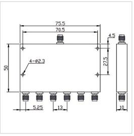
RF Solution offer a wide selection of 6 Ways Power Divider for global customers. PD06-F7650-S-6-18GHz is a 6 Ways Power Divider in Frequency Range of  $6.0{\sim}18.0$  GHz. It is made of high quality materials under a high standard, the Insertion Loss Max of this product is 1.8 dB, Isolation Min is 18 dB and Amplitude Unbalance is  $\pm 0.8$  dB. The component has a good working performance and stability, it is ideal for handling a Forward Power of 20 W.
