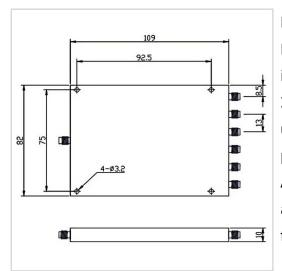
RF Solution offer a wide selection of 6 Ways Power Divider for global customers. PD06-F8211-S-2-18GHz is a 6 Ways Power Divider in Frequency Range of  $2.0 \sim 18.0$  GHz. It is made of high quality materials under a high standard, the Insertion Loss Max of this product is 2.2 dB, Isolation Min is 16 dB and Amplitude Unbalance is  $\pm 0.7$  dB. The component has a good working performance and stability, it is ideal for handling a Forward Power of 20 W.
