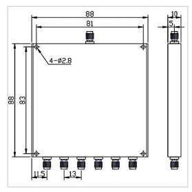
RF Solution offer a wide selection of 6 Ways Power Divider for global customers. PD06-F8888-S-1-4GHz is a 6 Ways Power Divider in Frequency Range of  $1.0{\sim}4.0$  GHz. It is made of high quality materials under a high standard, the Insertion Loss Max of this product is 1.5 dB, Isolation Min is 20 dB and Amplitude Unbalance is  $\pm 0.4$  dB. The component has a good working performance and stability, it is ideal for handling a Forward Power of 20 W.
