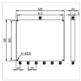
RF Solution offer a wide selection of 6 Ways Power Divider for global customers. PD06-F9214-S-0.8-18GHz is a 6 Ways Power Divider in Frequency Range of  $0.8{\sim}18.0$  GHz. It is made of high quality materials under a high standard, the Insertion Loss Max of this product is 4.0 dB, Isolation Min is 16 dB and Amplitude Unbalance is  $\pm 0.8$  dB. The component has a good working performance and stability, it is ideal for handling a Forward Power of 20 W.
