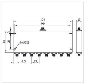
RF Solution offer a wide selection of 8 Ways Power Divider for global customers. PD08-F1040-S-6-40GHz is a 8 Ways Power Divider in Frequency Range of  $6.0{\sim}40.0$  GHz. It is made of high quality materials under a high standard, the Insertion Loss Max of this product is 2.0 dB, Isolation Min is 16 dB and Amplitude Unbalance is  $\pm 0.5$  dB. The component has a good working performance and stability, it is ideal for handling a Forward Power of 10 W.
