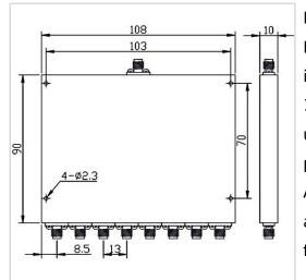
RF Solution offer a wide selection of 8 Ways Power Divider for global customers. PD08-F1190-S-1-4GHz is a 8 Ways Power Divider in Frequency Range of  $1.0 \sim 4.0$  GHz. It is made of high quality materials under a high standard, the Insertion Loss Max of this product is 1.5 dB, Isolation Min is 18 dB and Amplitude Unbalance is  $\pm 0.5$  dB. The component has a good working performance and stability, it is ideal for handling a Forward Power of 20 W.
