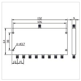
RF Solution offer a wide selection of 8 Ways Power Divider for global customers. PD08-F1364-S-2-4GHz is a 8 Ways Power Divider in Frequency Range of  $2.0\sim4.0$  GHz. It is made of high quality materials under a high standard, the Insertion Loss Max of this product is 1.0 dB, Isolation Min is 20 dB and Amplitude Unbalance is  $\pm0.4$  dB. The component has a good working performance and stability, it is ideal for handling a Forward Power of 20 W.
