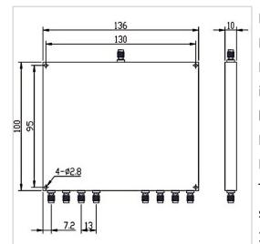
RF Solution offer a wide selection of 8 Ways Power Divider for global customers. PD08-F1410-S-1-12.4GHz is a 8 Ways Power Divider in Frequency Range of  $1.0 \sim 12.4$  GHz. It is made of high quality materials under a high standard, the Insertion Loss Max of this product is 3.5 dB, Isolation Min is 15 dB and Amplitude Unbalance is  $\pm 0.8$  dB. The component has a good working performance and stability, it is ideal for handling a Forward Power of 20 W.
