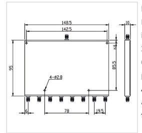
RF Solution offer a wide selection of 8 Ways Power Divider for global customers. PD08-F1595-S-2-18GHz is a 8 Ways Power Divider in Frequency Range of  $2.0 \sim 18.0$  GHz. It is made of high quality materials under a high standard, the Insertion Loss Max of this product is 3.0 dB, Isolation Min is 18 dB and Amplitude Unbalance is  $\pm 0.8$  dB. The component has a good working performance and stability, it is ideal for handling a Forward Power of 20 W.
