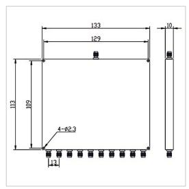
RF Solution offer a wide selection of 10 Ways Power Divider for global customers. PD10-F1311-S-800-4200MHz is a 10 Ways Power Divider in Frequency Range of  $800\sim4200$  MHz. It is made of high quality materials under a high standard, the Insertion Loss Max of this product is 2.5 dB, Isolation Min is 18 dB and Amplitude Unbalance is  $\pm 1.0$  dB. The component has a good working performance and stability, it is ideal for handling a Forward Power of 20 W.
