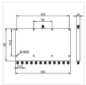
RF Solution offer a wide selection of 12 Ways Power Divider for global customers. PD12-F1692-S-4-10GHz is a 12 Ways Power Divider in Frequency Range of  $4.0\sim10.0$  GHz. It is made of high quality materials under a high standard, the Insertion Loss Max of this product is 2.2 dB, Isolation Min is 18 dB and Amplitude Unbalance is  $\pm0.5$  dB. The component has a good working performance and stability, it is ideal for handling a Forward Power of 20 W.
