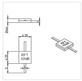
RF Solution offer a wide selection of Leaded Attenuator for global customers. RFT20N-60AM6363-6 is a Leaded Attenuator in Frequency Range of DC $\sim$ 6.0 GHz. It is made of high quality materials under a high standard, the Attenuation Value of this product is 20 dB, Attenuation Tolerance is  $\pm 0.8$  dB and VSWR Max is 1.25. The component has a good working performance and stability, it is ideal for handling a Rated Power of 60 W.
