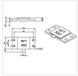
RF Solution offer a wide selection of Flanged Termination for global customers. RFT50-1000TM4826 is a Flanged Termination in Frequency Range of DC~1.0 GHz. It is made of high quality materials under a high standard, the Resistance Range of this product is 50  $\Omega$ , Resistance Tolerance is  $\pm 5\%$  and VSWR Max is 1.20. The component has a good working performance and stability, it is ideal for handling a Power of 1000 W.
