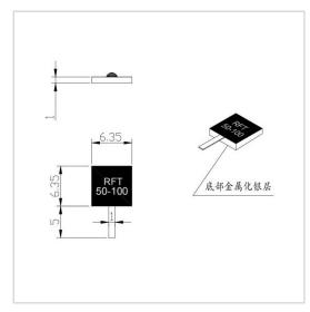
RF Solution offer a wide selection of Leaded Termination for global customers. RFT50-100TJ6363 is a Leaded Termination in Frequency Range of DC $\sim$ 6.0 GHz. It is made of high quality materials under a high standard, the Resistance Range of this product is 50  $\Omega$ , Resistance Tolerance is  $\pm 5\%$  and VSWR Max is 1.25. The component has a good working performance and stability, it is ideal for handling a Power of 100 W.
