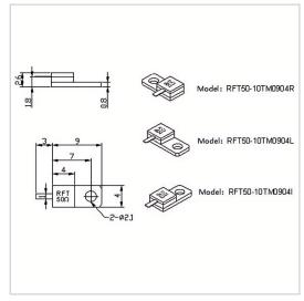
RF Solution offer a wide selection of Flanged Termination for global customers. RFT50-10TM0904 is a Flanged Termination in Frequency Range of DC~8.0 GHz. It is made of high quality materials under a high standard, the Resistance Range of this product is 50  $\Omega$ , Resistance Tolerance is  $\pm 5\%$  and VSWR Max is 1.20. The component has a good working performance and stability, it is ideal for handling a Power of 10 W.
