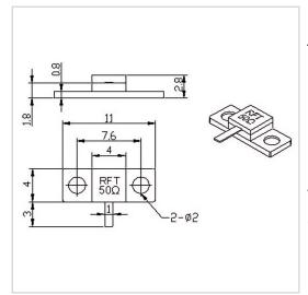
RF Solution offer a wide selection of Flanged Termination for global customers. RFT50-10TM1104 is a Flanged Termination in Frequency Range of DC~8.0 GHz. It is made of high quality materials under a high standard, the Resistance Range of this product is 50  $\Omega$ , Resistance Tolerance is ±5% and VSWR Max is 1.20. The component has a good working performance and stability, it is ideal for handling a Power of 10 W.
