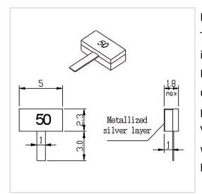
RF Solution offer a wide selection of Leaded Termination for global customers. RFT50-10TM5023 is a Leaded Termination in Frequency Range of DC~18.0 GHz. It is made of high quality materials under a high standard, the Resistance Range of this product is 50  $\Omega$ , Resistance Tolerance is ±5% and VSWR Max is 1.20~1.25. The component has a good working performance and stability, it is ideal for handling a Power of 10 W.
