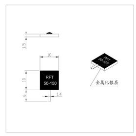
RF Solution offer a wide selection of Leaded Termination for global customers. RFT50-150TJ1010B is a Leaded Termination in Frequency Range of DC $\sim$ 6.0 GHz. It is made of high quality materials under a high standard, the Resistance Range of this product is 50  $\Omega$ , Resistance Tolerance is  $\pm 5\%$  and VSWR Max is 1.25 $\sim$ 1.30. The component has a good working performance and stability, it is ideal for handling a Power of 150 W.
