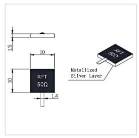
RF Solution offer a wide selection of Leaded Termination for global customers. RFT50-150TJ1010 is a Leaded Termination in Frequency Range of DC $\sim$ 3.0 GHz. It is made of high quality materials under a high standard, the Resistance Range of this product is 50  $\Omega$ , Resistance Tolerance is  $\pm 5\%$  and VSWR Max is 1.20. The component has a good working performance and stability, it is ideal for handling a Power of 150 W.
