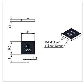
RF Solution offer a wide selection of Leaded Termination for global customers. RFT50-150TJ9595 is a Leaded Termination in Frequency Range of DC $\sim$ 3.0 GHz. It is made of high quality materials under a high standard, the Resistance Range of this product is 50  $\Omega$ , Resistance Tolerance is  $\pm 5\%$  and VSWR Max is 1.20. The component has a good working performance and stability, it is ideal for handling a Power of 100 W.
