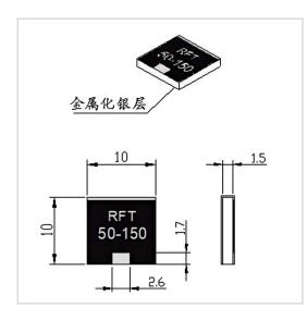
RF Solution offer a wide selection of Chip Termination for global customers. RFT50-150WT1010B is a Chip Termination in Frequency Range of DC $\sim$ 6.0 GHz. It is made of high quality materials under a high standard, the Resistance Range of this product is 50  $\Omega$ , Resistance Tolerance is  $\pm 5\%$  and VSWR Max is 1.25. The component has a good working performance and stability, it is ideal for handling a Power of 150 W.
