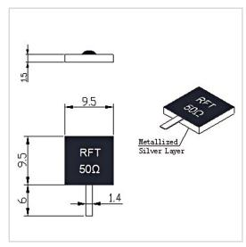
RF Solution offer a wide selection of Leaded Termination for global customers. RFT50-200TJ9595 is a Leaded Termination in Frequency Range of DC $\sim$ 3.0 GHz. It is made of high quality materials under a high standard, the Resistance Range of this product is 50  $\Omega$ , Resistance Tolerance is  $\pm 5\%$  and VSWR Max is 1.20. The component has a good working performance and stability, it is ideal for handling a Power of 200 W.
