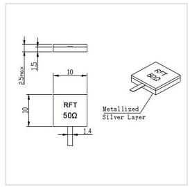
RF Solution offer a wide selection of Leaded Termination for global customers. RFT50-200TM1010 is a Leaded Termination in Frequency Range of DC $\sim$ 3.0 GHz. It is made of high quality materials under a high standard, the Resistance Range of this product is 50  $\Omega$ , Resistance Tolerance is  $\pm 5\%$  and VSWR Max is 1.20. The component has a good working performance and stability, it is ideal for handling a Power of 200 W.
