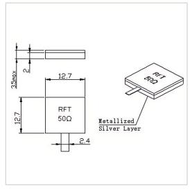
RF Solution offer a wide selection of Leaded Termination for global customers. RFT50-200TM1313B is a Leaded Termination in Frequency Range of DC~10.0 GHz. It is made of high quality materials under a high standard, the Resistance Range of this product is 50  $\Omega$ , Resistance Tolerance is  $\pm 5\%$  and VSWR Max is  $1.20\sim1.30$ . The component has a good working performance and stability, it is ideal for handling a Power of 200 W.
