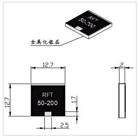
RF Solution offer a wide selection of Chip Termination for global customers. RFT50-200WT1313B is a Chip Termination in Frequency Range of DC $\sim$ 4.0 GHz. It is made of high quality materials under a high standard, the Resistance Range of this product is 50  $\Omega$ , Resistance Tolerance is  $\pm 5\%$  and VSWR Max is  $1.20\sim1.30$ . The component has a good working performance and stability, it is ideal for handling a Power of 200 W.
