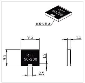
RF Solution offer a wide selection of Chip Termination for global customers. RFT50-200WT9595 is a Chip Termination in Frequency Range of DC $\sim$ 3.0 GHz. It is made of high quality materials under a high standard, the Resistance Range of this product is 50  $\Omega$ , Resistance Tolerance is  $\pm 5\%$  and VSWR Max is 1.20. The component has a good working performance and stability, it is ideal for handling a Power of 200 W.
