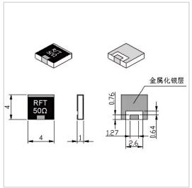
RF Solution offer a wide selection of Chip Termination for global customers. RFT50-20CT0404 is a Chip Termination in Frequency Range of DC $\sim$ 10.0 GHz. It is made of high quality materials under a high standard, the Resistance Range of this product is 50  $\Omega$ , Resistance Tolerance is  $\pm 5\%$  and VSWR Max is  $1.20\sim1.30$ . The component has a good working performance and stability, it is ideal for handling a Power of 20 W.
