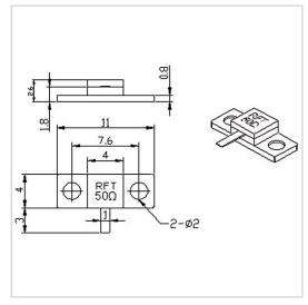
RF Solution offer a wide selection of Flanged Termination for global customers. RFT50-20TM1104 is a Flanged Termination in Frequency Range of DC $\sim$ 8.0 GHz. It is made of high quality materials under a high standard, the Resistance Range of this product is 50  $\Omega$ , Resistance Tolerance is  $\pm 5\%$  and VSWR Max is 1.20. The component has a good working performance and stability, it is ideal for handling a Power of 20 W.
