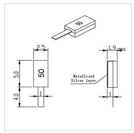
RF Solution offer a wide selection of Leaded Termination for global customers. RFT50-20TM2550 is a Leaded Termination in Frequency Range of DC~4.0 GHz. It is made of high quality materials under a high standard, the Resistance Range of this product is 50  $\Omega$ , Resistance Tolerance is  $\pm 5\%$  and VSWR Max is 1.20. The component has a good working performance and stability, it is ideal for handling a Power of 20 W.
