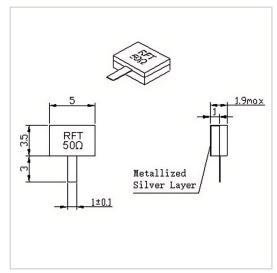
RF Solution offer a wide selection of Leaded Termination for global customers. RFT50-20TM5035 is a Leaded Termination in Frequency Range of DC~10.0 GHz. It is made of high quality materials under a high standard, the Resistance Range of this product is 50  $\Omega$ , Resistance Tolerance is  $\pm 5\%$  and VSWR Max is 1.20~1.25. The component has a good working performance and stability, it is ideal for handling a Power of 20 W.
