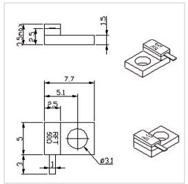
RF Solution offer a wide selection of Flanged Termination for global customers. RFT50-20TM7750 is a Flanged Termination in Frequency Range of DC $\sim$ 4.0 GHz. It is made of high quality materials under a high standard, the Resistance Range of this product is 50  $\Omega$ , Resistance Tolerance is  $\pm 5\%$  and VSWR Max is 1.20. The component has a good working performance and stability, it is ideal for handling a Power of 20 W.
