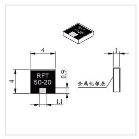
RF Solution offer a wide selection of Chip Termination for global customers. RFT50-20WT0404 is a Chip Termination in Frequency Range of DC $\sim$ 8.0 GHz. It is made of high quality materials under a high standard, the Resistance Range of this product is 50  $\Omega$ , Resistance Tolerance is  $\pm 5\%$  and VSWR Max is 1.20. The component has a good working performance and stability, it is ideal for handling a Power of 20 W.
